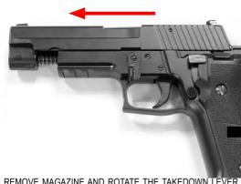
REMOVE MAGAZINE AND ROTATE THE TAKEDOWN LEVER CLOCKWISE UNTIL IT STOPS AND REMOVE THE SLIDE.
