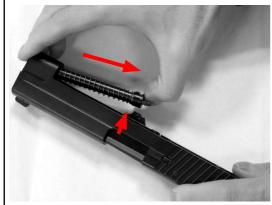
REMOVE THE RECOIL SPRING GUIDE AND SPRING.
